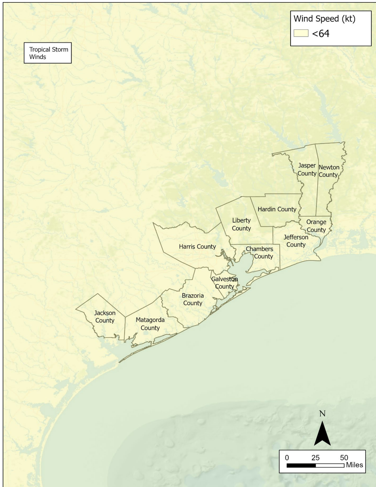
Figure 1-24 Wind Extent Map for Tropical Storm (60 kt) with 24 kt Forward Speed (Shaded Map)
